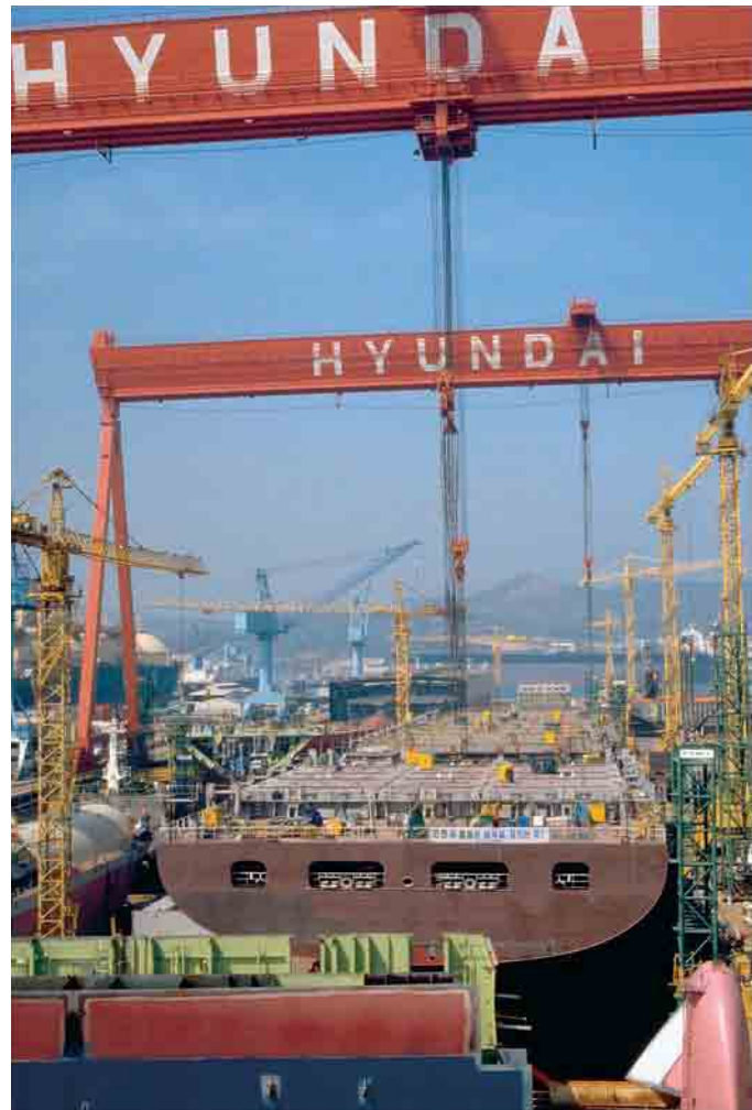
FIGURE 5.26 South Korea: Ulsan City Shipyard. The Hyundai chaebol is a major builder of large ships. Note the space required for assembling the materials and the range of equipment used in construction. Photo: © Vander Zwalm Dan/Corbis.
