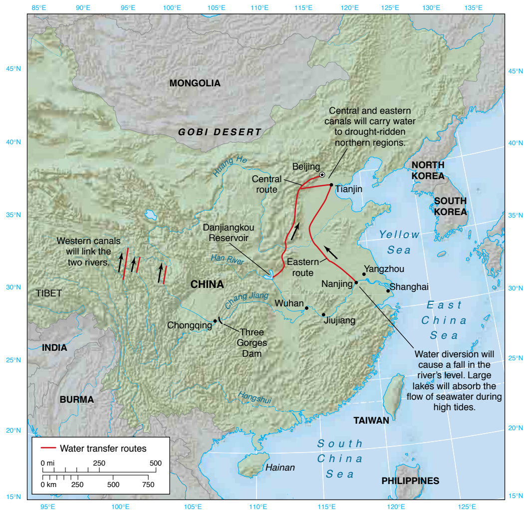
FIGURE 5.29 China: Potential Water Diversions. Northern China and the Huang He basin are increasingly short of water. Three potential diversions have been identified. The western routes are short, but mountainous, requiring tunnels; the central route requires a canal or aqueduct 1,240 km (770 mi.) long direct to Beijing; the eastern route follows existing channels, but their waters are polluted. Compare this map with the climate map, Figure 5.4, and the population map, Figure 5.14, to understand more fully the need for such diversions of water.
